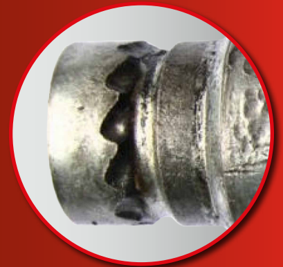
Brinelling on the male coupling
